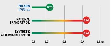
ASTM D4172. In 3rd party testing against 9 competitive products Polaris had 40% or better wear protection compared to all of the tested products. Numbers represent mm of wear scarring measured. Test measures wear at contact points, wear scar is measured for its length and width (in units of mm). Lower wear numbers mean better wear protection and friction reduction.
